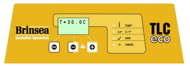
The TLC Eco control system utilises a highly accurate, calibrated sensor for temperature. Be cautious of low cost analogue or digital thermometers when comparing them with the brooder display readings.
