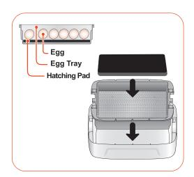
▶ Place eggs by adjusting tray divider according to egg size.
