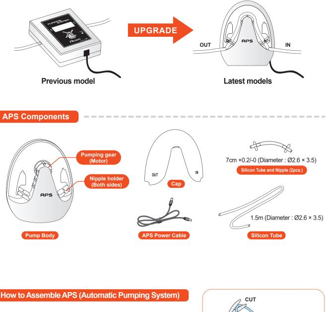
The silicone tube may become folded, causing a blockage. Please ensure that any blockages are removed by gentle pulling both ends of the tube before assembly.
