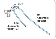
Cut the silicone tube to 1m and 0.5m lengths.
