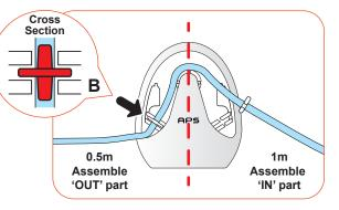
As shown in [Picture B], insert a nipple, attached to 0.5m silicone tube, into the 'OUT' part (left-hand side) of the nipple holder.
