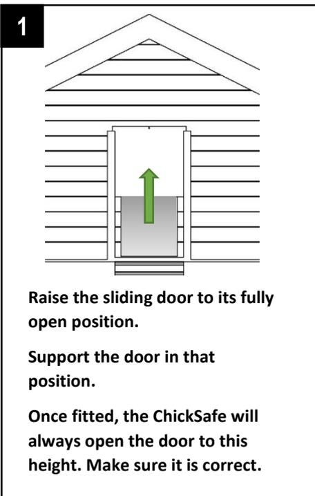
Raise the sliding door to its fully open position.
