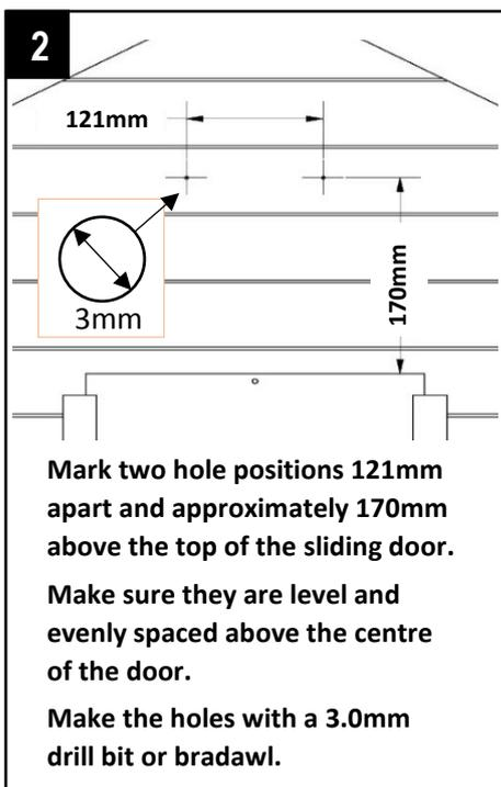
Mark two hole positions 121mm apart and approximately 170mm above the top of the sliding door.
