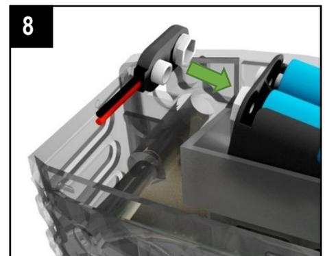
Fit the connector to the battery holder.
