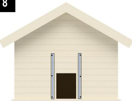
Position the channels on each side of the door hole on the hen house with the hole central between the channels. They must be perfectly vertical, flat and level. The fixing holes must be 322mm – 325mm apart.
