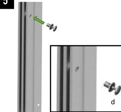
Fit a plastic rivet (d) to each channel in the hole shown.
