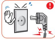
Do not use a damaged power cord or loose outlet.
