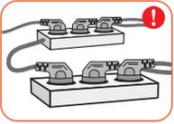
Do not insert multiple connecting plugs in an outlet.
