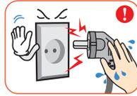
Do not pull the cord when taking out the power cord, and keep wet hands away from connecting plug.
